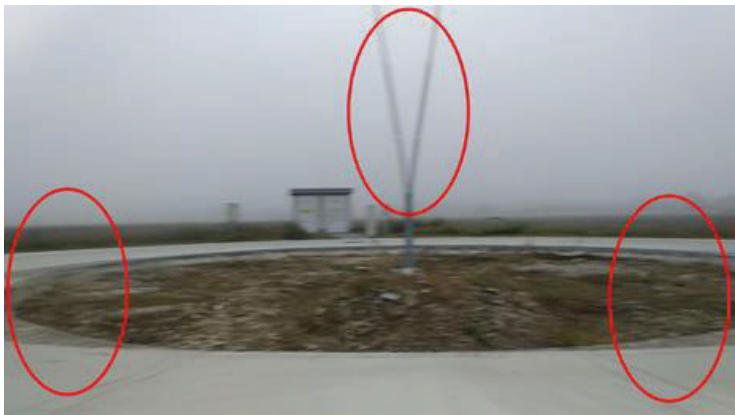
Fig. 9: In this created frame FE_3 is clearly seen how inadequate number of feature points and their layout in input frames creates double-exposure.
