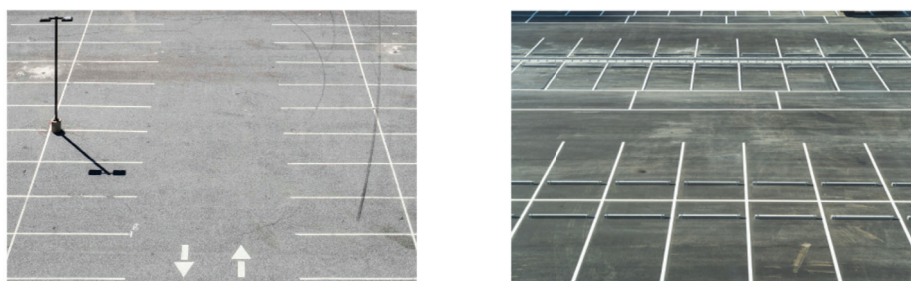
Fig. 3. Example of inappropriate (left) and appropriate (right) layout of the parking places in the camera view.
