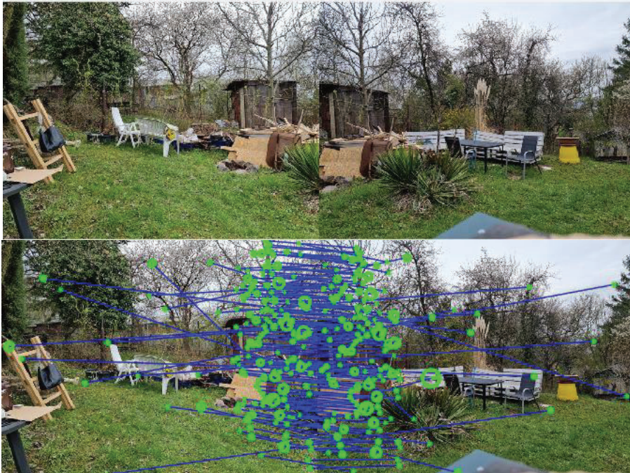
Fig. 5 – Example of feature matching. Upper image - initial image pair. Lower image - image pair with detected and matched SIFT features
